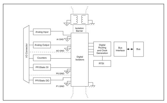
Figure 9-1. General NI 6232/6233 Block Diagram
